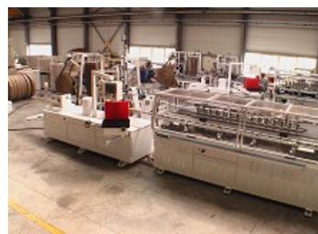
LIGNE DE SPIRALAGE HAUTE VITESSE, POUR LA FABRICATION DE CORPS DE BOÎTE EN CARTON
