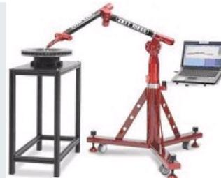
BRAS ARTICULÉ DE MESURE 6 AXES : MMT TRANSPORTABLE
