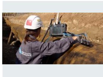
CONTRÔLE NON DESTRUCTIF PAR PHASED ARRAY SUR UN PIPELINE
