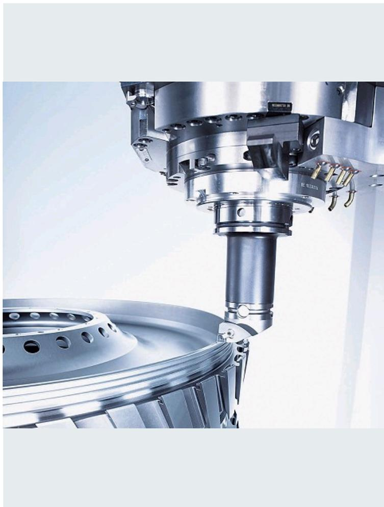
LES PRODUITS SINUMERIK ET SINAMICS SONT CONÇUS POUR GÉRER LES MACHINES-OUTILS MULTITECHNOLOGIQUES. CI-DESSUS UNE FRAISEUSE SACHANT TOURNER, ÉQUIPÉE D'UN AXE B, D'UNE TABLE ROTATIVE AINSI QUE D'UNE CAPACITÉ DE GESTION DES OUTILS DE TOURNAGE.
