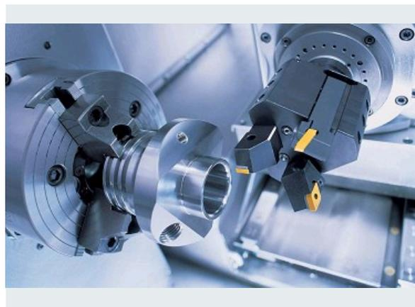
CI-DESSUS UN TOUR SACHANT FRAISER, AXE Y ET AXE B PERMETTANT TOUTES LES OPERATIONS DE FRAISAGE SUR PLAN INCLINÉ.
