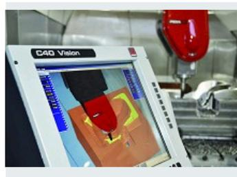
VIMILL® LOGICIEL DE SIMULATION USINAGE ET ANTI-COLLISION 5 AXES
