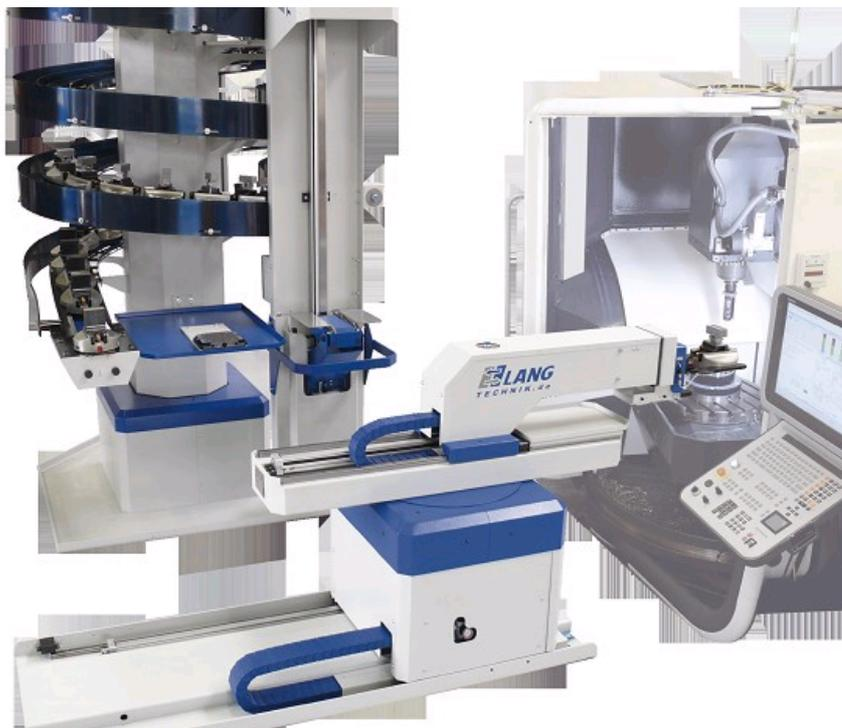
LE SYSTÈME AUTOMATION ECOTOWER PERMET D'ALIMENTER AUTOMATIQUEMENT EN PIÈCES LA GRANDE MAJORITÉ DES CENTRES D'USINAGE 3, 4 OU 5 AXES. IL S'INSTALLE SUR MACHINES NEUVES OU EN RETROFIT SUR MACHINES EXISTANTES
