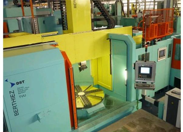
TOURS VERTICAUX DE 800 À 2500 MM, HAUTE PRESSION 400 BAR, TOURNAGE, FRAISAGE, RECTIFICATION, PALETTISATION
