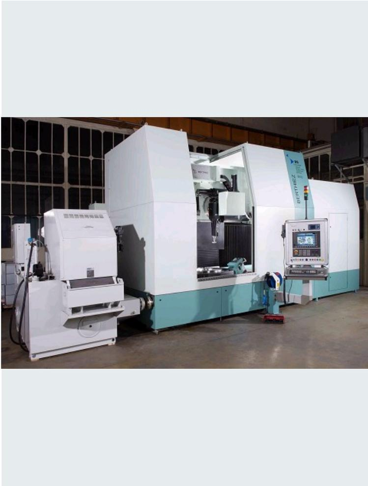
RECTIFIEUSES VERTICALES DE 800 À 6000 MM, PLATEAU HYDROSTATIQUE, ENTRAÎNEMENT DIRECT PAR MOTEUR COUPLE, ÉLECTROBROCHES DE 7 À 45 KW, TOURNAGE DUR
