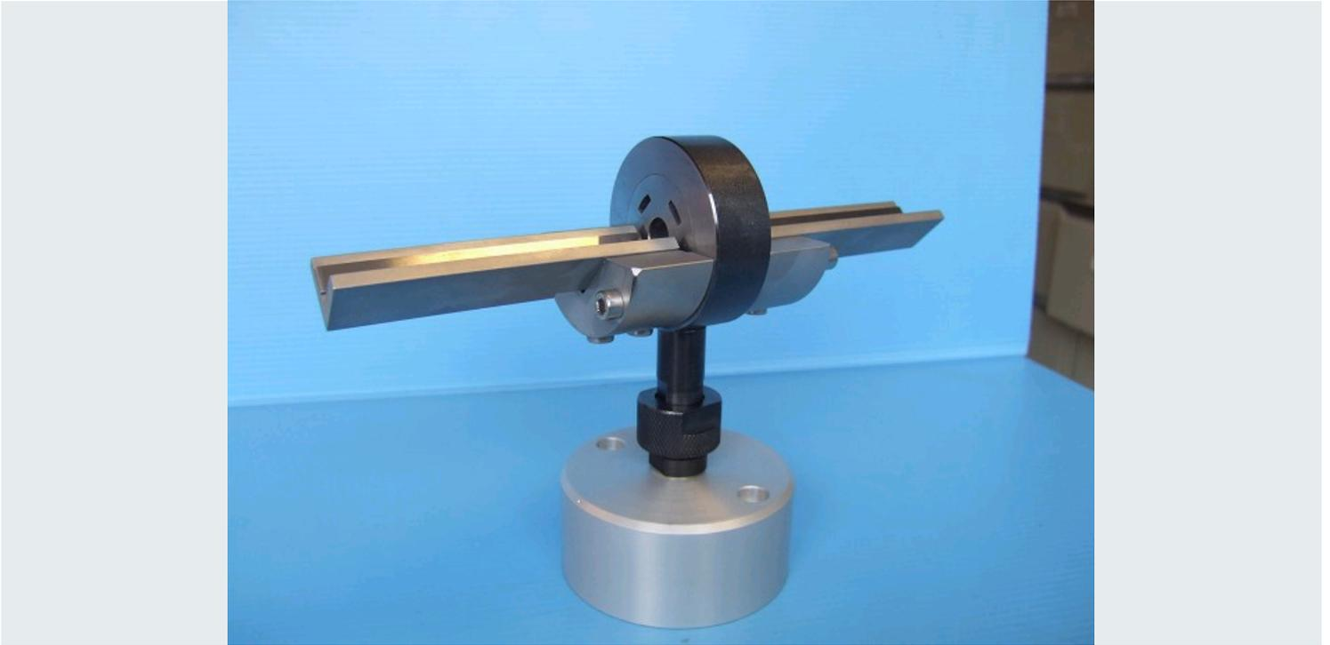
BAGUE DE MESURE PNEUMATIQUE AVEC VÉS
