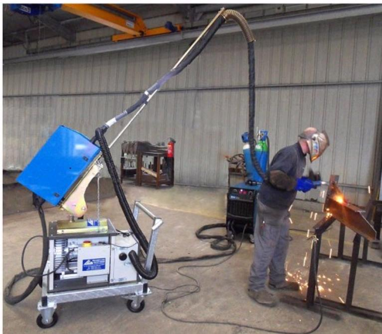
ENGMAR PROPOSE DES SOLUTIONS DE CAPTAGE, FILTRATION ET REJET DES FUMÉES DE SOUDAGE / COUPAGE.
